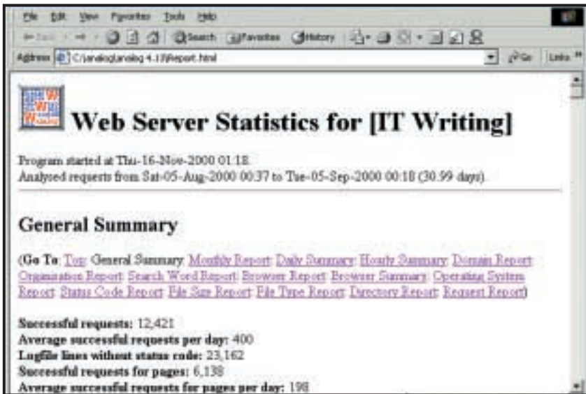
The Analog report is an HTML file with sections indexed by hyperlinks
